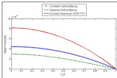
**Figure 4: Axial Force Versus Normalized Length**
