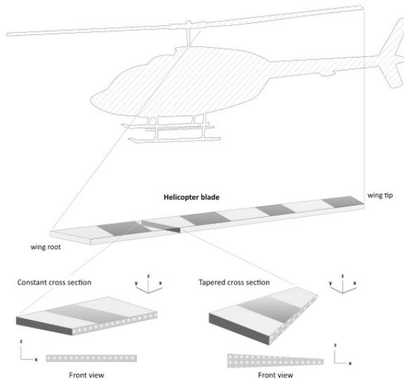
Figure 1: Bell 206 JetRanger with Constant- and Tapered-Cross-Section Blades. [2]
