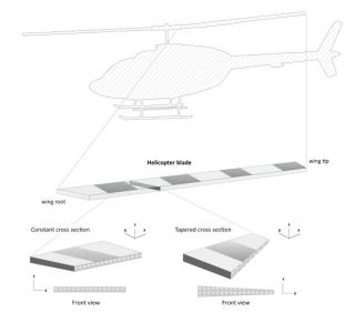
Figure 1: Bell 206 JetRanger with Constant- and Tapered-Cross-Section Blades. [2]
