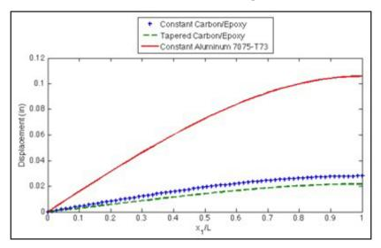
Figure 3: Displacement Versus Normalized Length.
